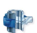
在公接头密封表面装有O型橡胶环以便密封更严密。可用型号采用对焊Sch.40。 推荐用于歧管和管道连接,负压使用和腐蚀性使用场合。 O-shape rubber ring is mounted on the seal surface of the male connector for better sealing. Butt weld Sch.40 is desired for the applicable figure. It is recommended for connection of manifold and pipes and for applications with negative pressure and corrosion.
